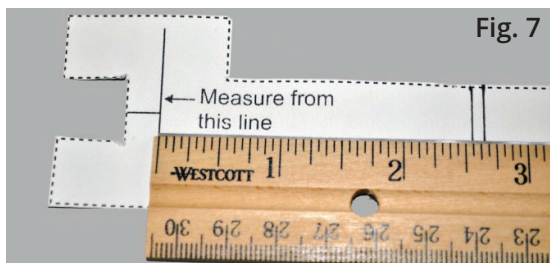
Fig. 7 Using a ruler, measure from the printed line to your marks. Measure these distances to the nearest 1/16" or millimeter.
